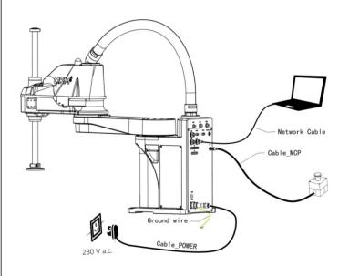
1. Install the network cable, ground wire, cable \_MCP and cable \_POWER according to the schematic diagram.
