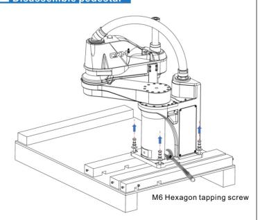
1. Use a adjustable wrench to remove the fixing screw.
